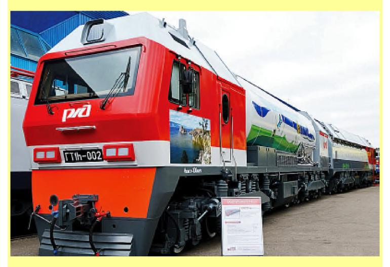
Russian Railways have agreed to test a new prototype locomotive built by Sinara Traction at their Production Plant in Lyudinovsky. This new locomotive has a Gas Turbine power unit which uniquely is fuelled by Liquified Natural Gas (LNG) which powers the turbine at high speed, all of which is then coupled to an electric generator supplied by YETM Privod, to generate electric current for the axle mounted traction motors.
